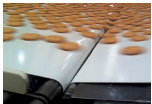
Standard TPU series Food. Highly resistant to animal and vegetable oils and fats, no cracks, high level of hygiene. High resistance to cut and abrasion. Fabrics with low capillarity (Wicking Test G11-FDA 2011).
