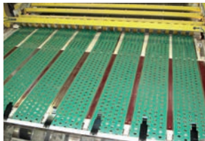
Hipro series Industry. Excellent resistance to abrasion, better than some elastomers, highly antistatic, fusion splice. Conveyance and processing of cardboard, paper and other abrasive materials.
