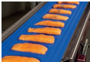
Premium TPU series Food. Bacteriostatic formulation with strong and long lasting antimicrobial & antibiofilms effects (ISO 22196). Highly resistant to hydrolisis. Fabrics with low capillarity (Wicking Test G11-FDA 2011).
