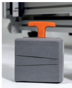
Photo of the 90x10 cutting head and belt sample with single fingers.
