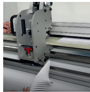
Photo of the 90x10 cutting head and belt sample with single fingers.
