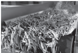
Washflow series Food. High resistance plastic mesh belts. A new concept in belts for the washing and conveyance of vegetables, fruit and frozen food, as well as for draining liquids and screening solid waste.
