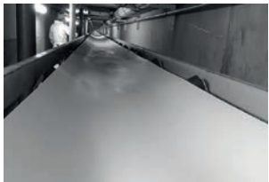
Febor series Industry. Green – Packaged or grain products free of oils or fats. Black – Flame retardant belts, airports, logistics centres. Food. White and blue - FDA food-quality, flame-retardant, resist. to abrasion. Sugar, carrots and other vegetables.
