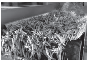
Washflow series Food. High resistance plastic mesh belts. A new concept in belts for the washing and conveyance of vegetables, fruit and frozen food, as well as for draining liquids and screening solid waste.
