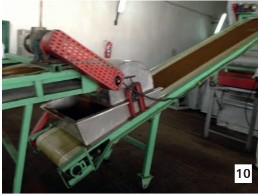
10 to 12. After fermentation the brown tea is transferred to the Dryer on a Clina 20CK/Clina 21CK, Clina 2035, Clina 12CF or Clina 20CF belt.
