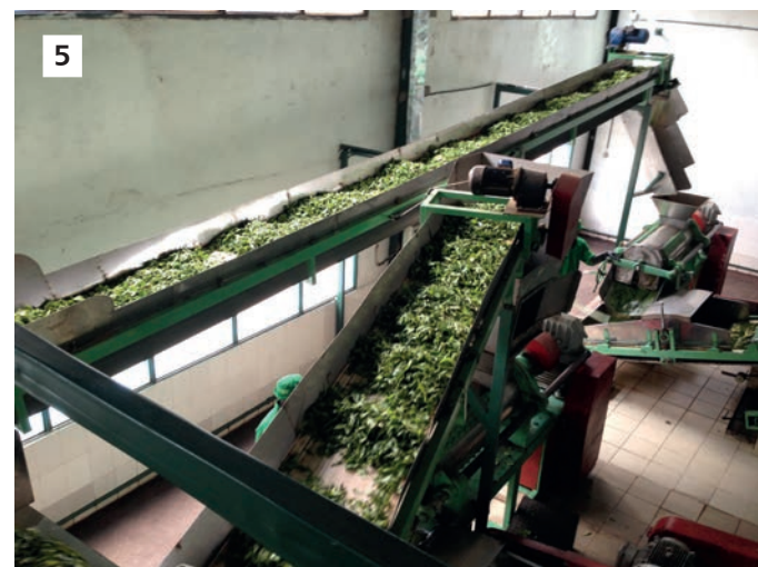
5. Incline conveyor from lines 1 and 2 to C.T.C. belt ( Clina 12CF ).
