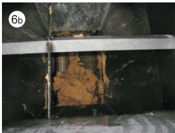
6b The off-cut falls into the hopper to be reused.
