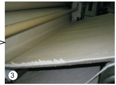
3 Different sheets until the desired thickness is obtained. PU or cotton-polyester belts. They must be matt or "FF" to allow good transfer.
